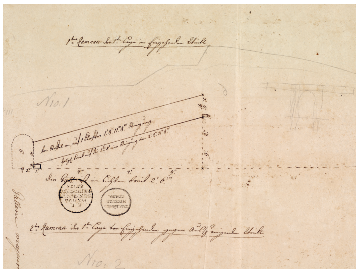
Layout plan for the establishment of level 1 mine branches No. 1, featuring a sketch of the rampart line and the construction principle (VHA, undated – 1780s).
